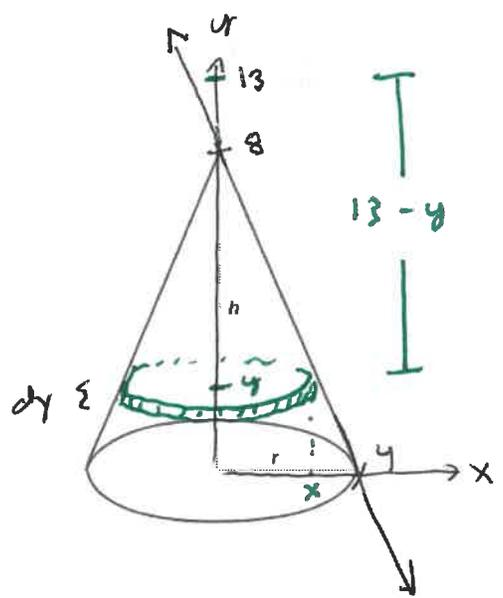
$$\begin{aligned} d\text{Area} &= \pi x^2 \\ d\text{volume} &= \pi x^2 dy \\ d\text{mass} &= 1000 \pi x^2 dy \\ d\text{force} &= 1000(9.8) \pi x^2 dy \\ d\text{work} &= 1000(9.8) \pi x^2 (13-y) dy \end{aligned}$$
