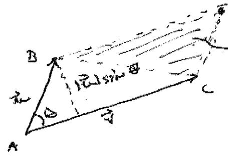
Area of triangle is  $\frac{1}{2}$  the area of the parallelogram.  $= \frac{|\vec{u}| |\vec{v}| \sin \theta}{2}$
